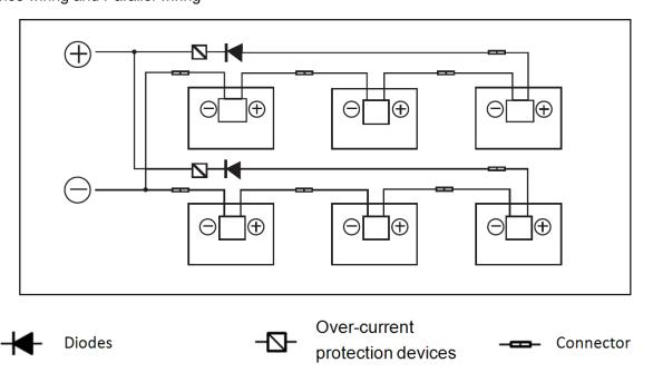
Figure 11: Electrical Diagrams of Series and Parallel Wiring
