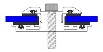
Figure 3 Cross-section structure of clamp
