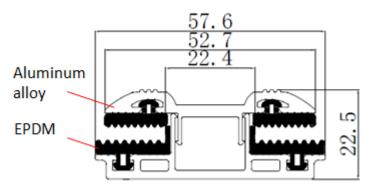
Figure 1-b Clamp structure (only for frameless bifacial mono PERC glass-glass module)
