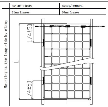
Figure 8 Installation Position and Corresponding Load Relationship
