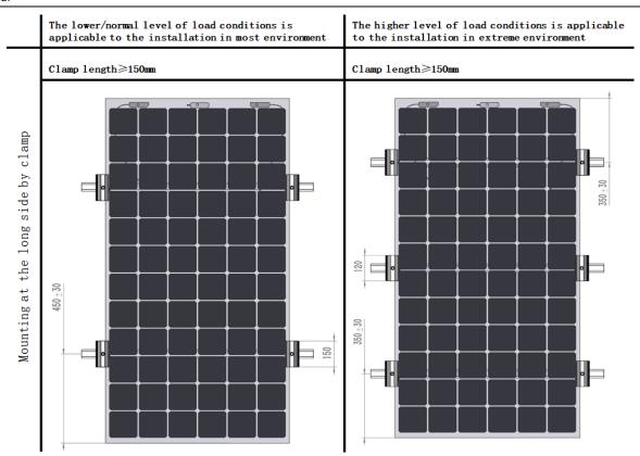
Figure 5-a Position requirements for clamps installation of 72 double glass modules
