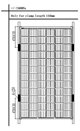
Figure 4-b Position requirements for clamps installation of 60 bifacial mono PERC glass-glass modules
