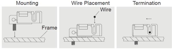
Screw Head Flush with Base; Wire Bottomed in Wire Slot Slider Covers Base; Base Flush with Frame Wire is Terminated
