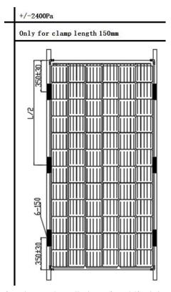
Figure 5-b Position requirements for clamps installation of 72 bifacial mono PERC glass-glass modules
