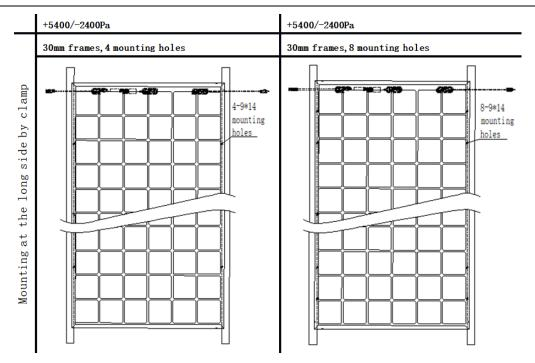
Figure 7 Installation Position and Corresponding Load Relation
