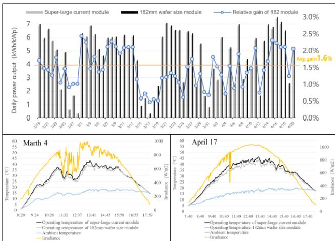
Figure 6. Comparison of Power Generation and Typical Daily Operating Temperature of Super-large Current Module and 182mm Wafer Size Module.
