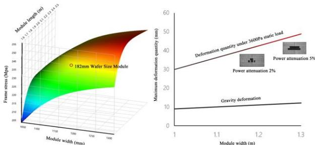
Figure 3. The mechanical loading capability of 182mm Wafer Size Module is within the safety limit. When the width of the module exceeds 1.2m, the deformation under load will bring micro-cracks and power degradation obviously.
