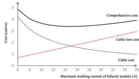
Figure 5. The curve diagram of relationship between the comprehensive cost (= cable cost + cable loss cost) of 4mm<sup>2</sup> cable and the maximum working current of bifacial module (superimposed on back side)
