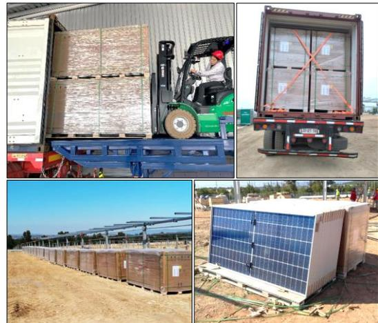
Figure 1. The 182mm Wafer Size Module is packaged in a horizontal way, which maximizes the utilization of container space and provides about 10cm of loading and unloading margin allowance. The module can be placed stably on the project site.
