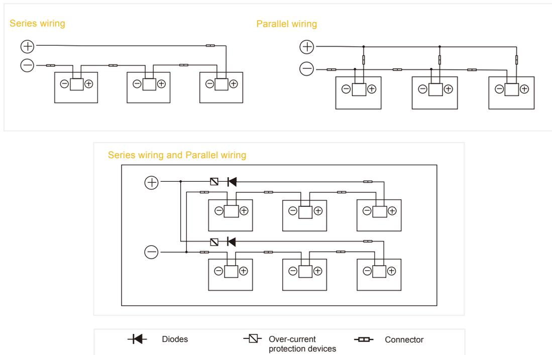
Figure 5: Electrical diagrams of series and parallel wiring
